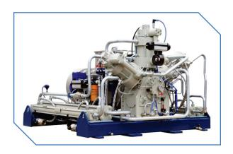
Suction pressure:  $1 \div 8$  bar Discharge pressure: 250 bar Installed power:  $75 \div 200$  KW N° cylinders / N° stages: 3 / 4 Body cylinders: single effect (SE)
